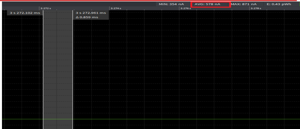
Figure 5: Deep sleep current measurement in Power measurement device(Otii Arc)
